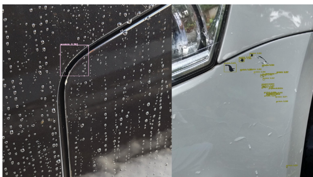
Fig. 12. Damage detection on surfaces with water.
