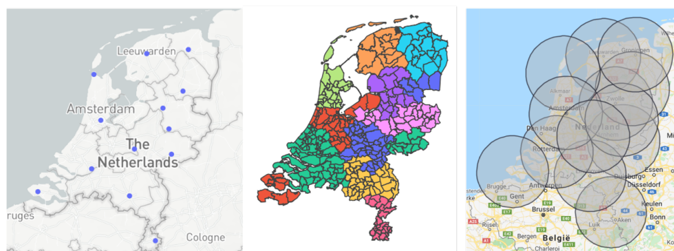
Figure 1. Verification of the placement of hubs by checking the maximum travel distance constraint (in this example 60 km).
