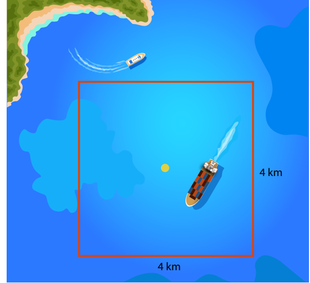
Figure 2. The defined range of the selected hydrophones to align raw PAM recordings with the AIS pulses.
