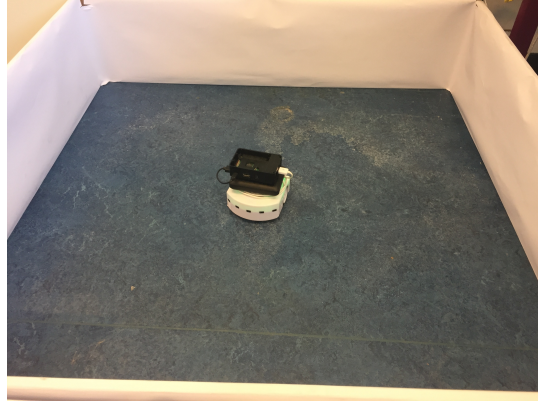
FIGURE 9.3: The environment with one robot for the obstacle avoidance task. This setup is duplicated for the number of robots used in the experiment.
