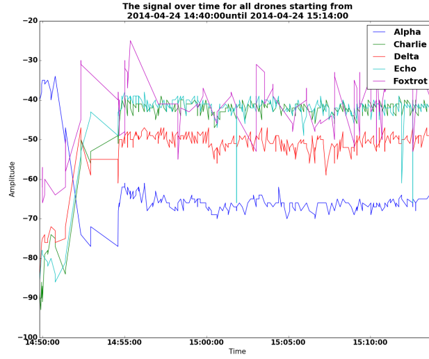
Figure 4.3: The signal strength of the five drones during the Test 1
