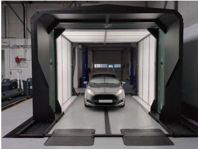
FIGURE 1. Drive-through vehicle inspection system which is completely enclosed to reduce influence from its surroundings.
